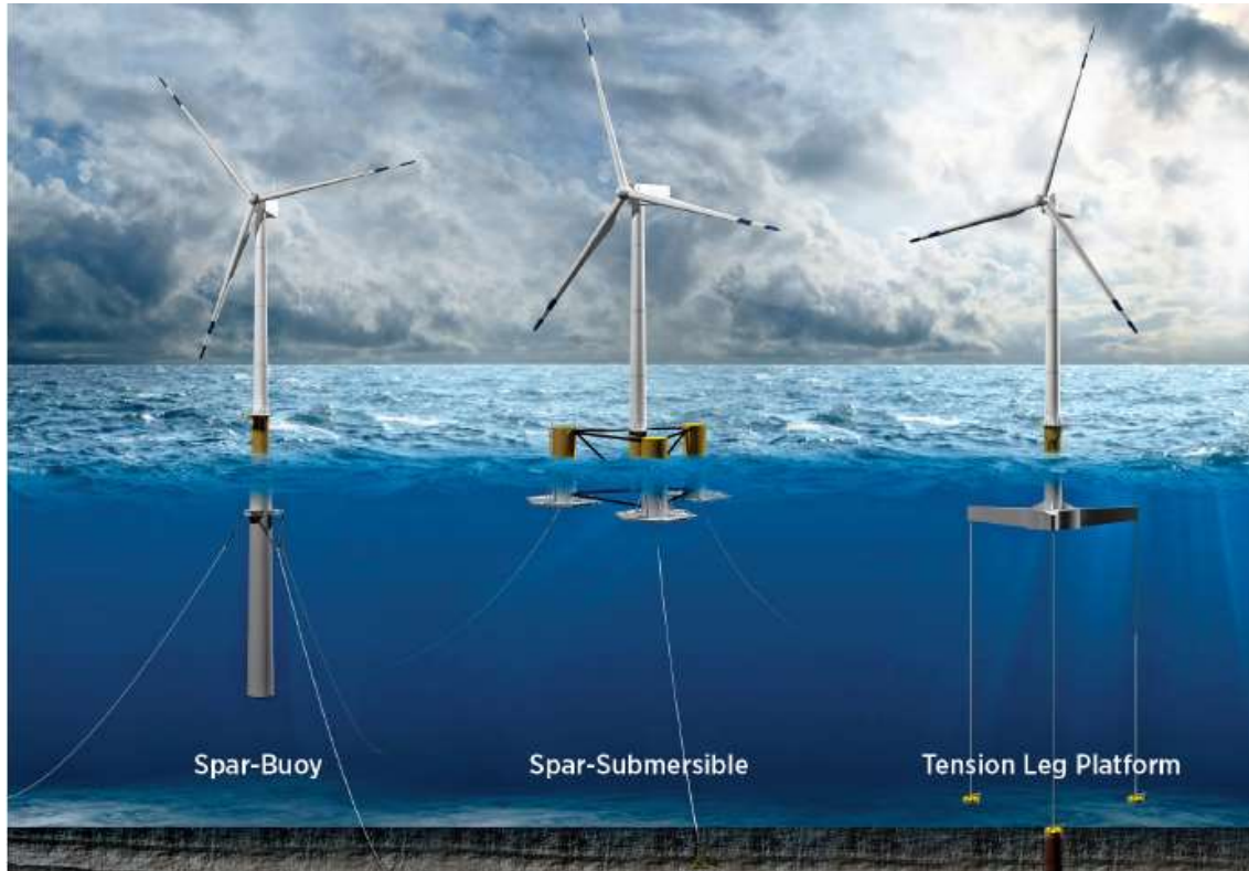
Figure 3: Types of platform for off-shore wind turbine (International Renewable Energy Agency (IRENA) 2016).
