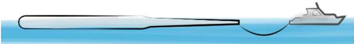
Figure 13: Towing of Windcrete.
