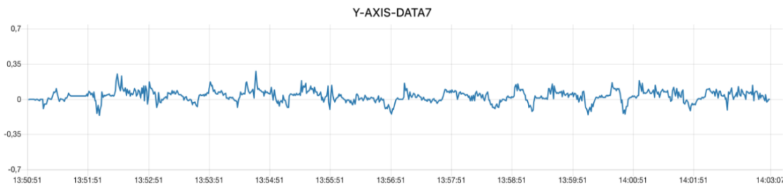
Figure 14: Result of the first filter script applied on the Data 7 Y-AXIS data, Y-axis is exposed in g's and the X-axis in time.
