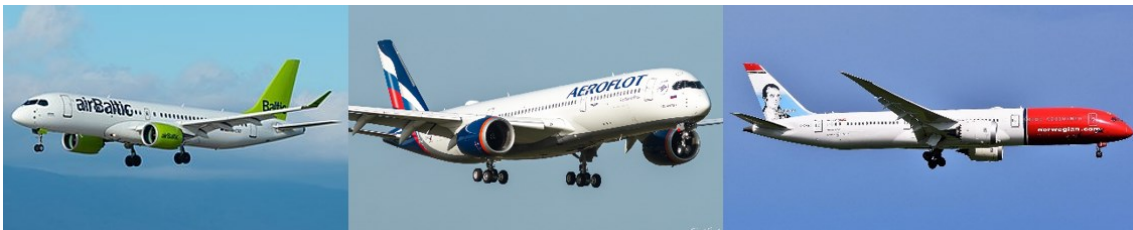
Fig. 3.1 Most modern aircraft by 2020. From left to right: Airbus A220-300 [11], Airbus A350 XWB [12], Boeing B787 [13]
