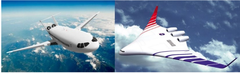
Fig. 3.2 Conventional concept aircraft. From left to right: Double Bubble D8 [14], NASA's blended wing body (BWB) concept [15]
