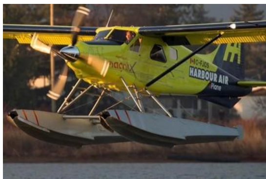
Fig. 3.7 DHC-2 modified with a fully electric power plant from harbour air. [36]
