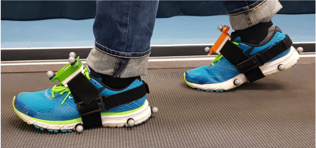
FIGURE 4.6: Setup of IMU and optical markers during the trials
