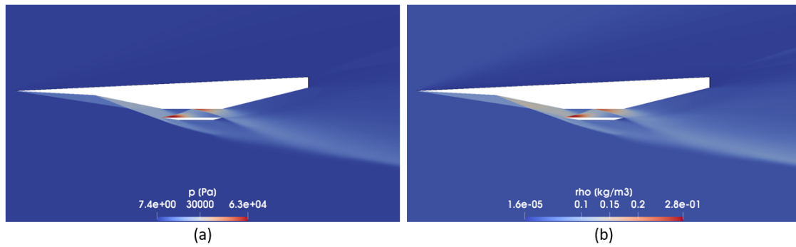
Figure 12. Pressure field (a) and density field (b) of case 1 for AoA = 14^\circ .
