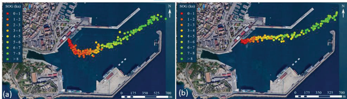
Figure 5. Ship position and Speed Over Ground (SOG) from AIS data at case study quay from August 1, 2018 to November 30, 2018. (a) Departure manoeuvres; (b) Arrival manoeuvres
