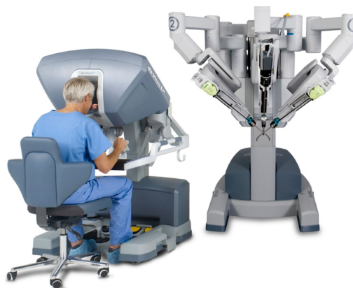
Figure 8: Robotic laparoscopy system da Vinci developed by Intuitive Surgical.
