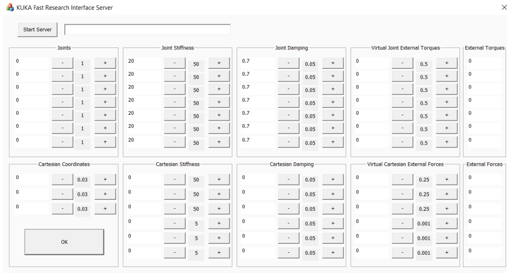
Figure 43: Graphic user interface simulating the KUKA LWR teach pendant using FRI. Available at the laboratory prior to this project.
