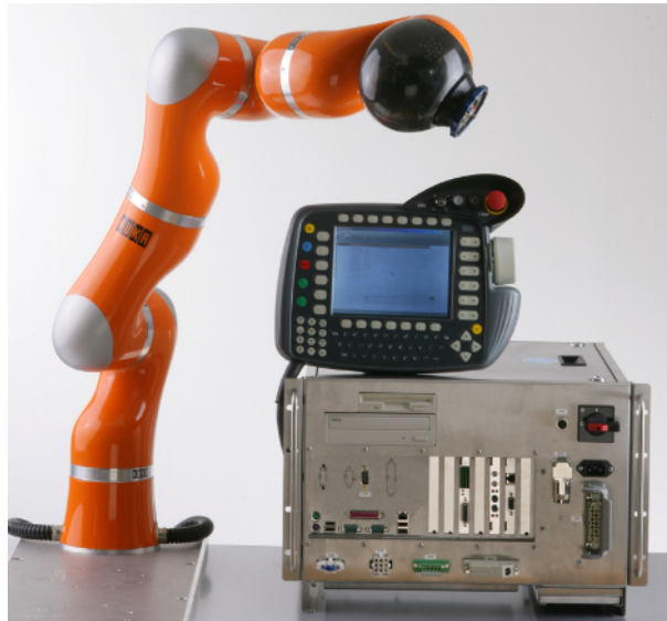
Figure 39: The Kuka LightWeight Robot 4 with KUKA Robot Controller (KRC) and KUKA control panel (KCP)
