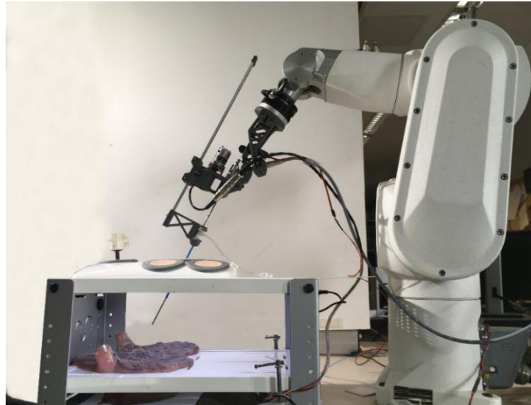
Figure 5: Slave module with current robot holding the fetoscope, Trocar Compensator and Laser Coagulation Module. A silicone placenta is placed on the MistraTrainer platform (by SurgiTrainer).
