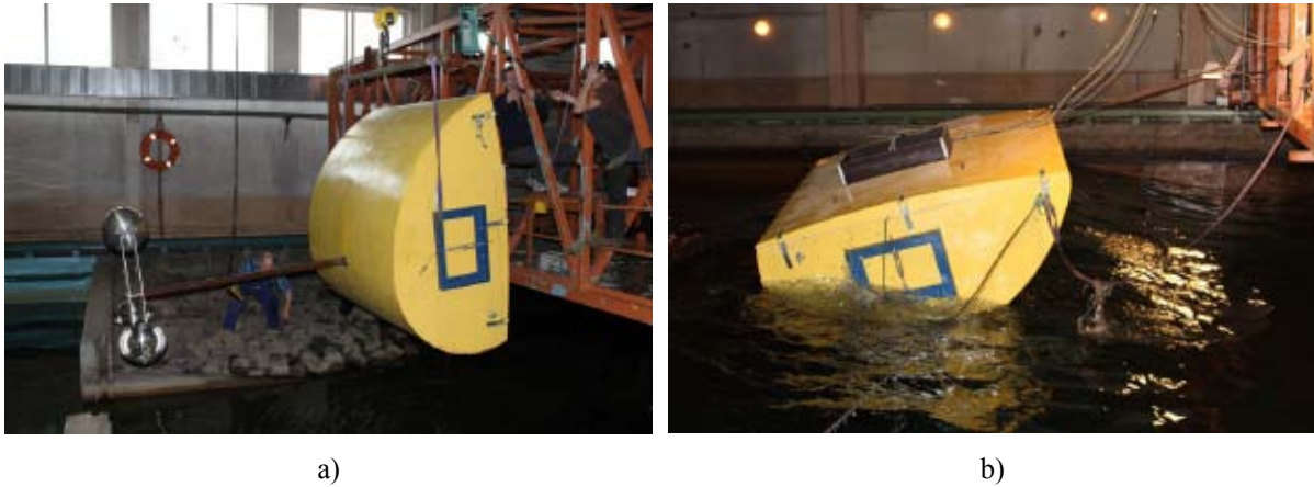
Figure 5: a) Preparations for model test; b) Enwrgr buoy during tests on regular wave
