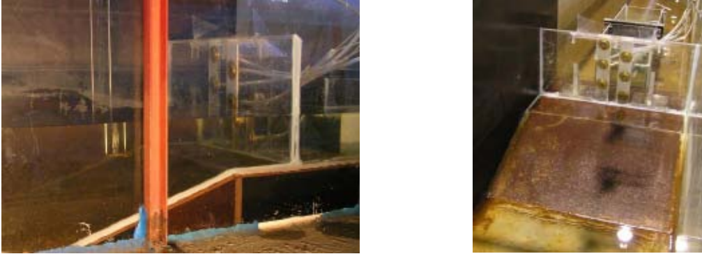
Figure 3: Physical breakwater model in the flume with position of the pressure sensors.
