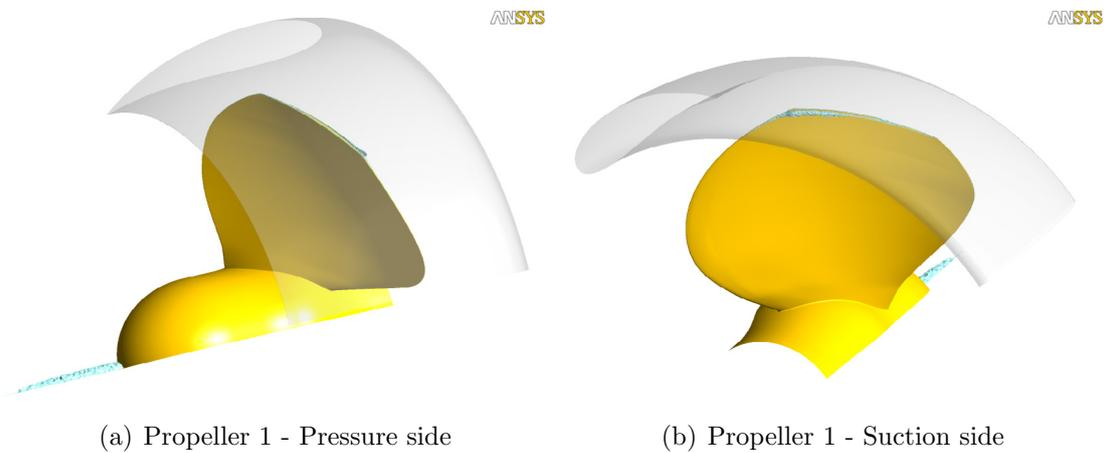
**Figure 2:** Cavitation on Propeller 1 by isosurfaces at  $C_p = -\sigma$ .
