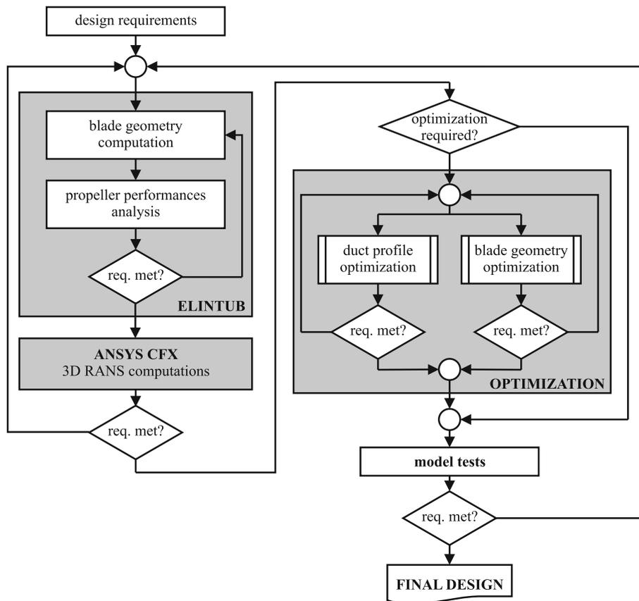
Figure 1: Ducted propeller design flow chart.
