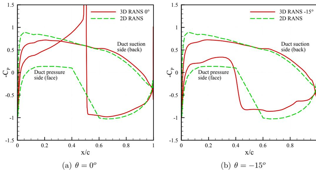
**Figure 4:** Comparison between 2D and 3D computed duct pressure distributions.
