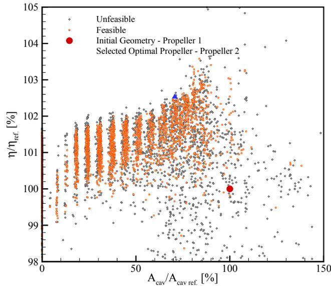
**Figure 3:** Pareto distributions of optimal geometries.
