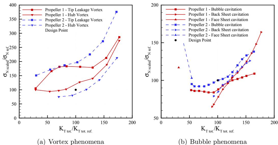
Figure 6: Normalized Cavitation Buckets.
