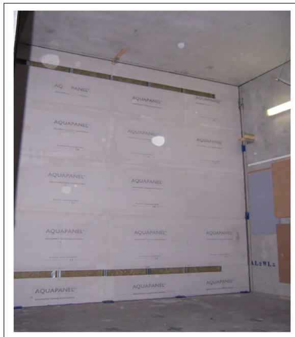
Figure 7. Photo inside the LARGE reverberation chamber, taken during the airborne sound insulation tests. The upper and lower ventilation openings can be distinguished.
