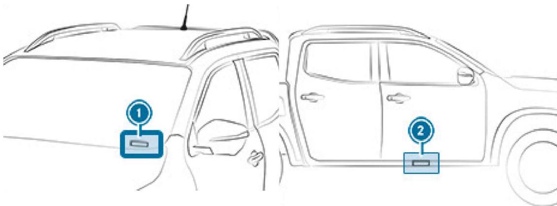
Figure 6. Vehicles' locations where VIN plates are usually placed.
