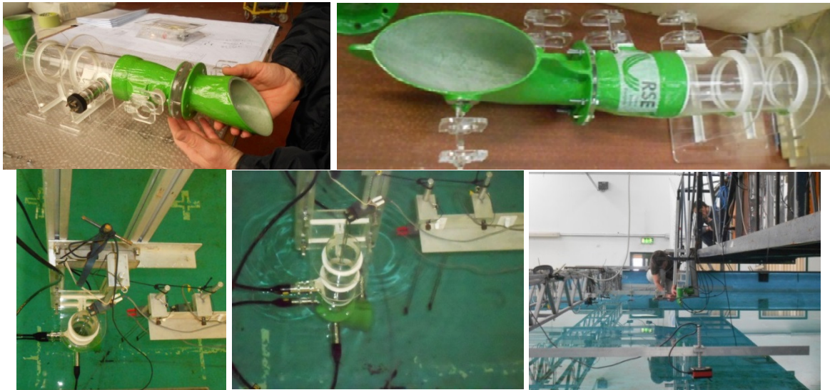
Figure 7: Laboratory tests (scale 1:20): Wavetube (up left) and Wavesax (up right). Device in the basin during the tests and position of the level and pressure sensors (down).
