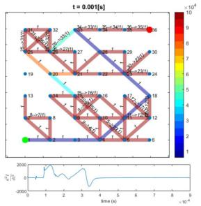
**Fig. 4** Visualization of the simulation results after 0.001s for an SPP computation concerning the search of a path from node 1 to 36 in a random directed graph defined on a 6×6 grid, while applying a voltage ramp rising from 0 to 100V in 1ms. Memristors were simulated using the memristor model of [19] with  $[R_{ON}, R_{OFF}] = [2, 200] K\Omega$  (see description in section 3). At the bottom, the evolution of the 2<sup>nd</sup> time derivative of the current is shown.
