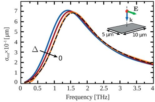
Fig. 3. Extinction cross section per unit width of a  $10 \mu\text{m}$  wide graphene patch with length  $L = 5 \mu\text{m}$ . Results of the surface impedance model (dashed black line) and the equivalent slab model (solid lines) are shown at room temperature ( $T = 300 \text{ K}$ ) and zero electrostatic bias ( $\mu_c = 0 \text{ eV}$ ). The thicknesses of the equivalent graphene slab  $\Delta$  are 500 nm, 200 nm and 5 nm, from left to right.
