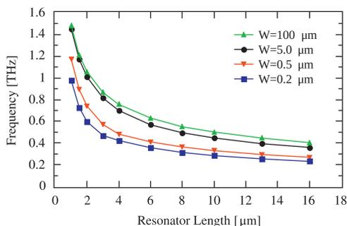
Fig. 6. Dependence of the first resonant frequency of the graphene antenna on its length,  $L$ , for different widths,  $W = 100 \mu\text{m}$ ,  $W = 5 \mu\text{m}$ ,  $W = 0.5 \mu\text{m}$  and  $W = 0.2 \mu\text{m}$ .
