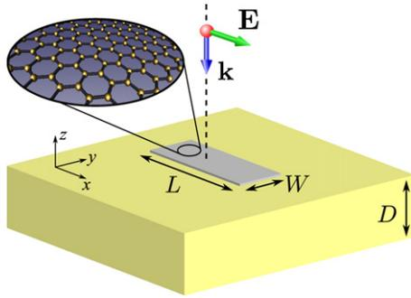
Fig. 1. Sketch of the graphene-based nano-antenna under consideration.
