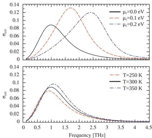
Fig. 8. Dependence of the antenna resonant frequency on the electrostatic bias at  $T = 300$  K (top) and on the temperature at  $\mu_c = 0$  eV (bottom).  $L = 1 \mu\text{m}$ ,  $W = 0.5 \mu\text{m}$ ,  $D = \infty$  and  $\epsilon = 11.9$ .
