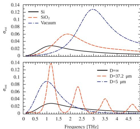
Fig. 7. Top: normalized extinction cross section of the graphene antenna placed on different substrates, silicon ( $\epsilon=11.9$ ), silica ( $\epsilon=4.0$ ) and vacuum (left to right). Bottom: normalized extinction cross section for different thickness of silicon substrates,  $D = \infty$  (solid),  $D = 37.5 \mu\text{m}$  (dashed) and  $D = 5 \mu\text{m}$  (dashed-dotted).
