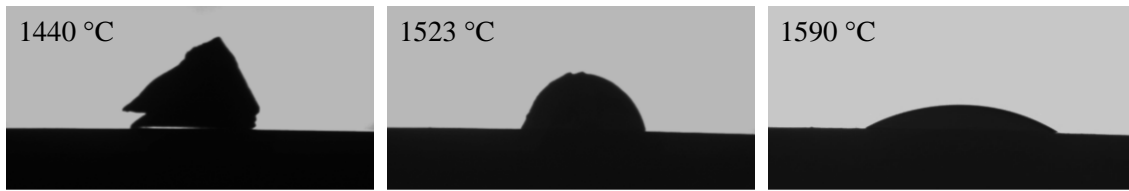
Figure 5. Contact-angle adapted camera pictures taken at 1440, 1523 and 1590 °C, showing the metal drop formation and evolution for Fe 15 Ni 10 Cr-Ti(C,N) system.
