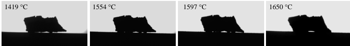
Figure 11. Fe 10 Cr 10 Al-Ti(C,N) contact-angle adapted camera pictures taken at different temperatures, showing the no-formation of the metal drop.
