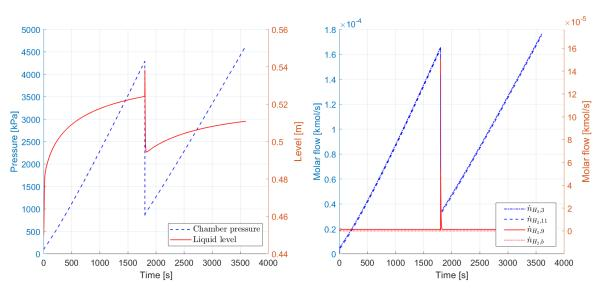
Figure 3: Model response in the H<sub>2</sub> separation chamber to a valve opening.
