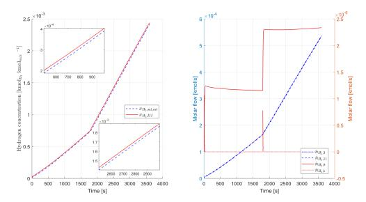
Figure 4: Model response in the H<sub>2</sub> separation chamber to a electric current input change.
