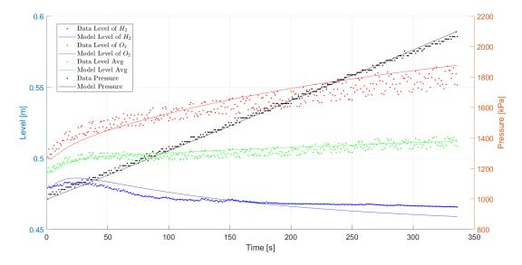
Figure 5: Comparison of pressurization between the real system (dotted line) and the model (solid line). In this case, the electrolyzer is operating with output values closed.
