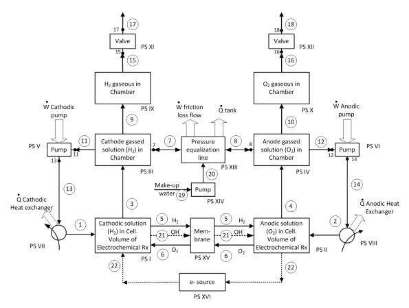
Figure 2: Flow diagram with the PSs numbered in Roman. Mass flows are identified with numbers within circles
