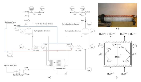
**Figure 1:** (a) Piping and instrumentation diagram of the ELH, (b) real cell package, and (c) scheme of the electrolytic cell with reactions.  $H_2O^{(*)}$  represents KOH solution and  $O_2^{(**)}$  and  $H_2^{(**)}$  represent outputs that are contaminated with H<sub>2</sub> and O<sub>2</sub>, respectively.
