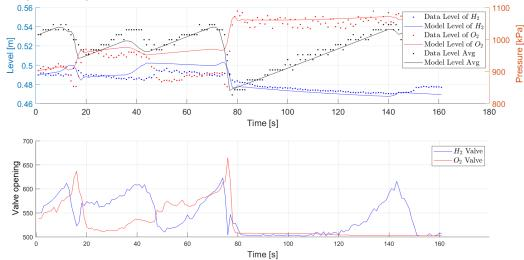
Figure 6: Upper figure: comparison of normal operation at 1000 kPa between the real system (dotted line) and the model response (solid line). In the lower figure it can be seen the opening valves, above  $u_{min} = 600$  the valve is open.
