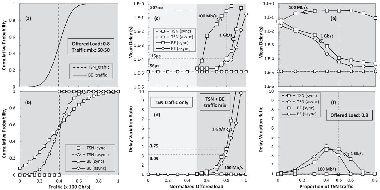
Fig. 4. Performance of TSN and BE traffic when they are mixed on a common network interface
