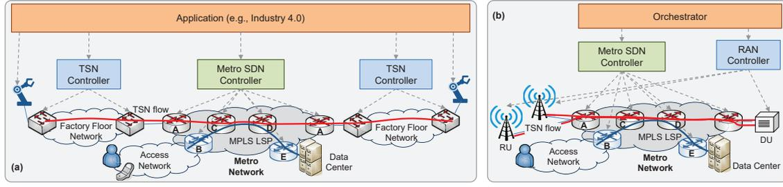
Fig. 1. Illustrative architectures supporting TSN and BE traffic over a Metro network. TSN traffic from Industry 4.0 (a) and RAN fronthaul (b).
