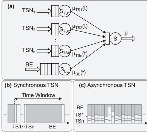
Fig. 2. Modeling TSN and BE traffic mixing
