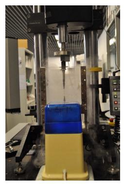
**Figure 3.** Experimental setup. Instron Microtester 5548 System with two clamps holding the sample. The samples are subjected to the tensile test under a humidity-controlled environment to prevent sample drying.
