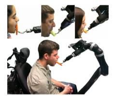
Figure 1: The Jaco robot feeding users using different manipulation strategies. Source: [9]
