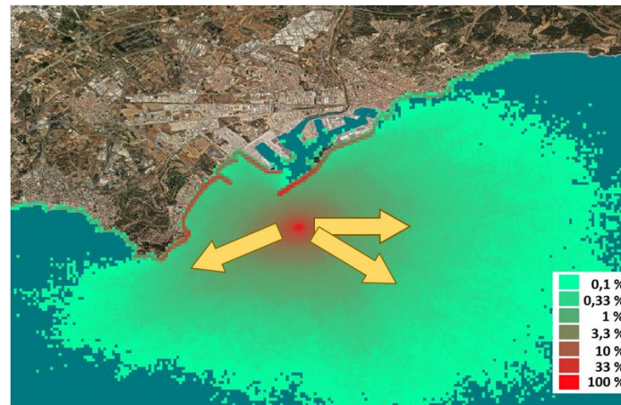
Figure 5. Main directions for oil spills from the monobuoy. Yellow arrows show the main direction of dispersion of a potential oil spill based on probability maps.
