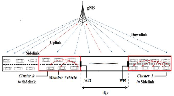
Fig. 1. The system model of the cellular network with sidelink V2V.
