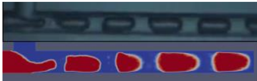
Fig. 5.2 Bubble generation comparison between the experiments and the simulations for the U_{SG} = U_{SL} = 0.5 \text{ m/s} case
