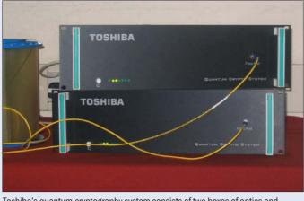
Toshiba's quantum-cryptography system consists of two boxes of optics and electronics, which sit at two sites connected by optical fibre and are designed to fit inside standard communications racks. All data fed into one unit are encrypted and transmitted via the fibre to the unit at the other site, where they are decrypted.
