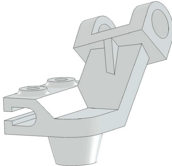
Figure 5. This is an example of a part with a nerve whose placement would be much easier if based on the bisecting plane concept.
