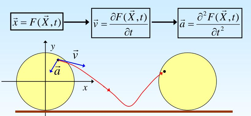
$$\begin{vmatrix} x = r\omega & t + R\cos(\Theta - \omega t) \\ y = R\sin(\Theta - \omega t) \end{vmatrix} v_x = r\omega + R\omega\sin(\Theta - \omega t)$$
