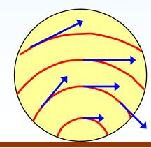
**Streamlines** are found by seeking the field lines of the field  $\vec{v}(\vec{x},t)$  at a given t i.e., by solving the system of ODE in the parameter s:
