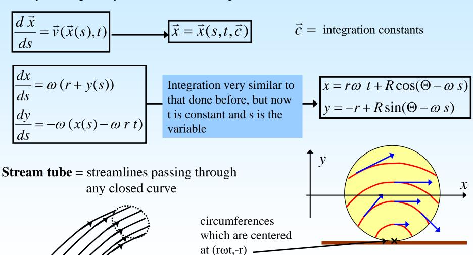
If the velocity field is steady, streamlines and path lines coincide
