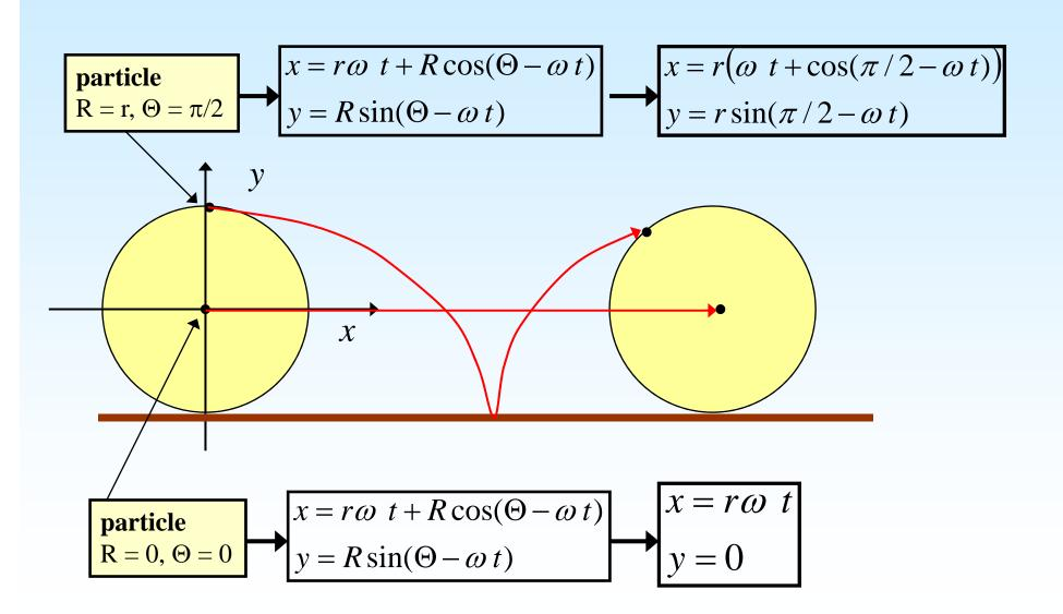
$(R, \Theta)$  = material or Lagrangian coordinates of the particle = label for each particle
