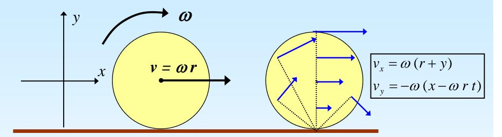
$$a_{x} = \frac{\partial v_{x}}{\partial t} + v_{x} \frac{\partial v_{x}}{\partial x} + v_{y} \frac{\partial v_{x}}{\partial y} = 0 + 0 - \omega^{2}(x - \omega rt)$$
