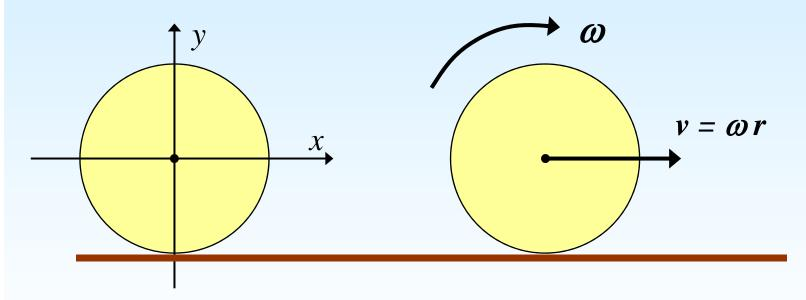
How to describe the motion of the particles?
