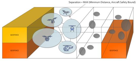
Figure 9. The Aircraft Safety Bound concept by DLR.
