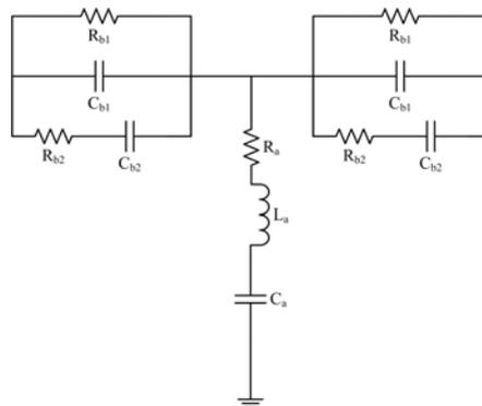
Figure 2. Impedance circuit based on RLC cell that models bulk impedance of samples and its undesired ground coupling.
