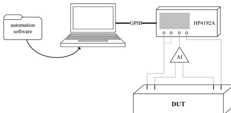
Figure 1. Schematic diagram of the complete instrumentation system performing 4-wire electrical impedance measurement on a 600x150x150 mm prismatic sample.
