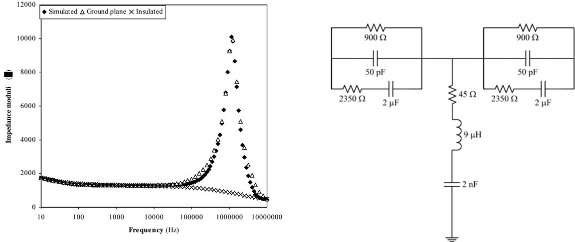
Figure 3. (a) Impedance moduli vs. frequency for sample measurements on ground plane triangles ( $\Delta$ ) trace, on an insulated environment crosses ( $\times$ ) trace and for simulated equivalent circuit rhombuses ( $\blacklozenge$ ) trace, and (b) simulated circuit agreeing with measured data.
