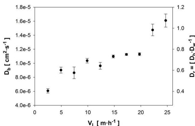
**Figure 3. Results of the average effective diffusivity (●) in a biofilm density of 21.20 g VSS<sup>-1</sup>·L<sup>-1</sup>, calculated from oxygenation profiles, at different flow velocities**
