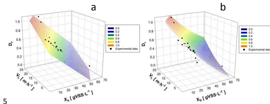
**Figure 4. Two different approaches for biofilm diffusivity estimation from liquid flow velocity and biofilm density. a) Linear multi-variable model, and b) general multi-variable model.**
