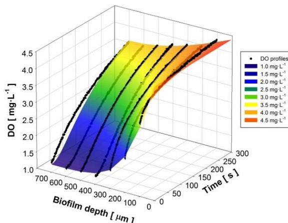
**Figure 1. Simulated (mesh) and experimental (circle) oxygenation profiles obtained in a single measurement used in the determination of diffusivity in a biofilm section.**
