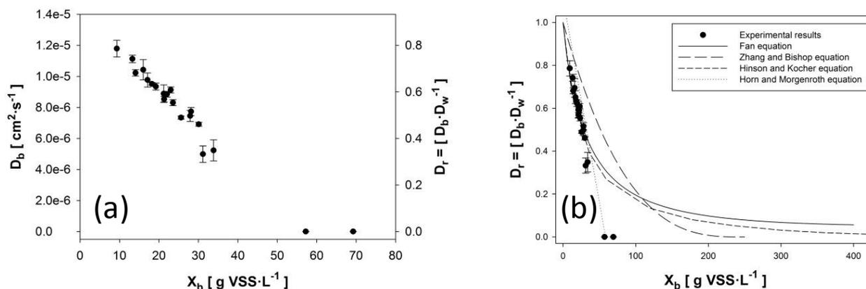
**Figure 2. (a) Oxygen diffusivity ( $D_b$ ) and biofilm diffusivity ( $D_r$ ) in function of biofilm densities. The experiments were performed operating the reactor at a flow velocity of 9.88 m·h<sup>-1</sup>. (b) Biofilm diffusivities measured at different biomass densities versus different available correlations for biofilm diffusivity estimation.**
