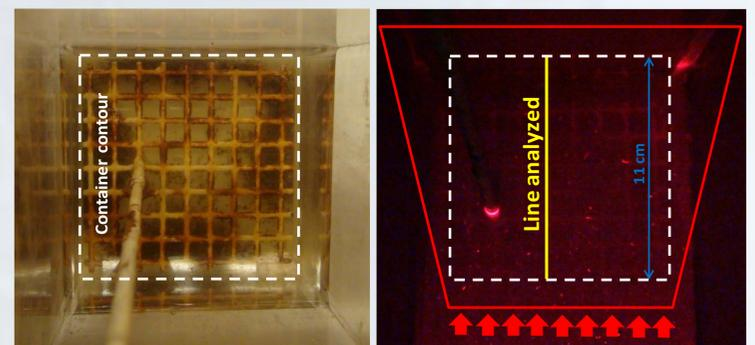
**Fig 1.** Left: Image of the grid with biosolids. Right: Image obtained indicating the laser projection, the container contour and the line analyzed.
