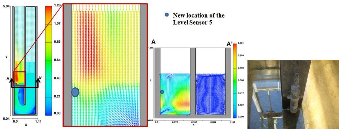
**Figure 10:** New location of the Level Sensor 5.
