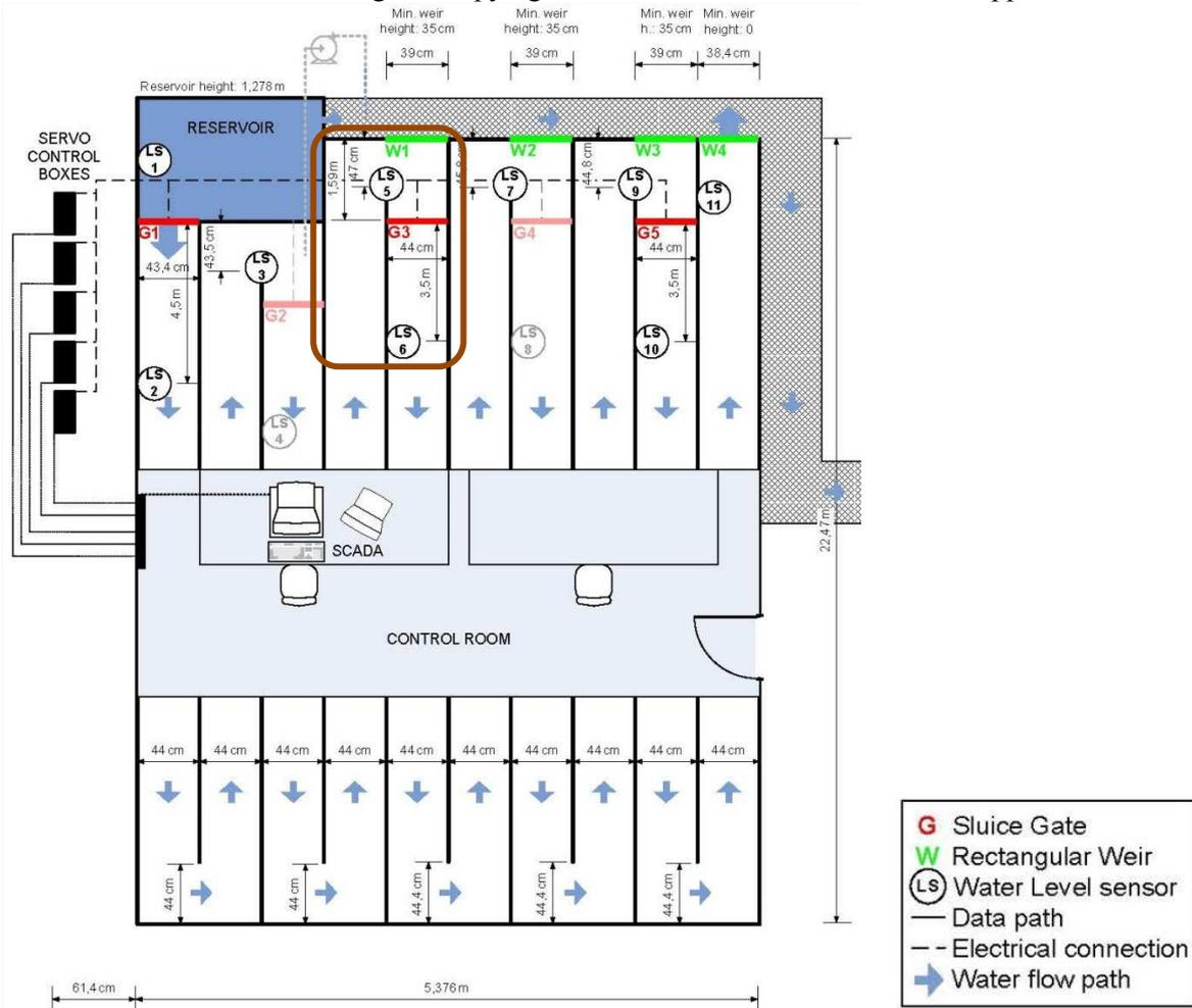
Figure 2: Detailed scheme of the whole PAC-UPC canal.
