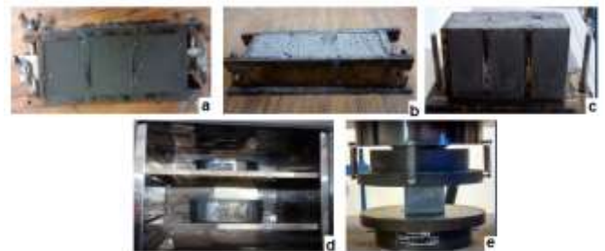
Figure 1. Experiment performed. a) Processing specimens, b) Specimen ready for stripping, c) Unmold specimens, d) Curing chamber, e) Compression test specimens.
