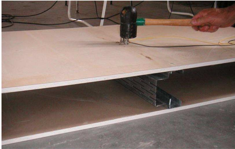
Figure 16: Picture of the location of a stud between the leaves [24].
