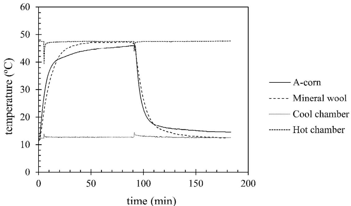
Figure 2: Dynamic thermal behaviour. Internal temperature for A-corn sample is compared with a mineral wool.
