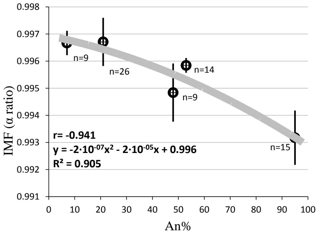
**Figure 2.** Proposal of regression line for the plagioclase standards composition and the IMF ( $\alpha$  ratio). Error bars represent standard deviation.  $n$  is the number of used points for calculation;  $r$  is Pearson's linear correlation coefficient;  $y$  is Best fitted equation and  $R^2$  is best fitting coefficient.
