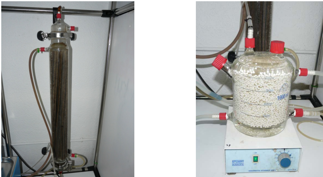
Fig. 4. View of the continuous reactors one week after inoculation. Left: up-flow reactor filled with polyester non-woven material. Right: perfectly stirred reactor packed with PVA gel beads.
