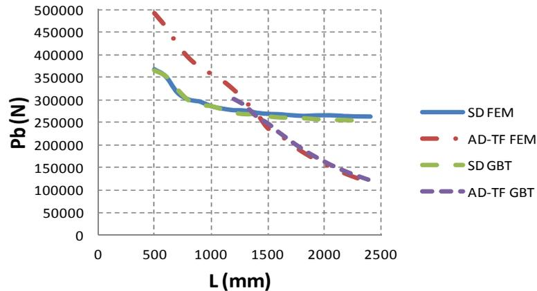
Figure 2. Result of a linear buckling analysis (SD: symmetric distortional buckling; AD-TF: anti-symmetric distortional buckling - torsional-flexural buckling; FEM: Finite Element Method; GBT: Generalised Beam Theory).
