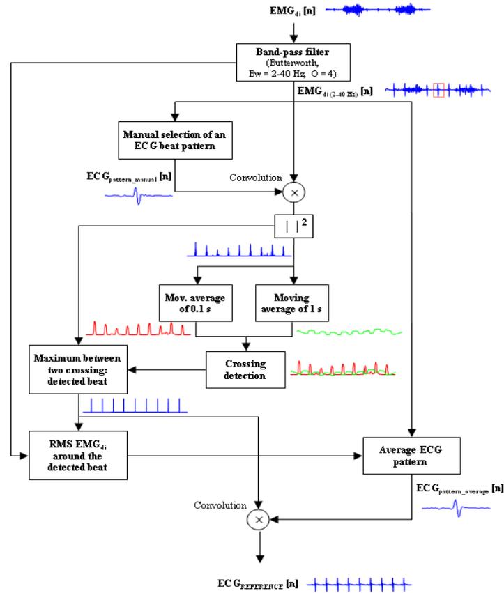
Fig 3 Block diagram of the algorithm for detection and estimation of the ECG activity present in the EMG<sub>di</sub> signal (ECG reference)
