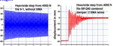
Study of the 50 m length cable of IFSTTAR. Left: free oscillation. Right: Damped behavior by SMA. The SMA damper reduces the displacement amplitude over time.
