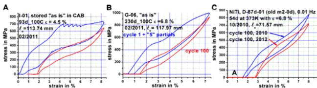
Temperature-stress aging in NiTi. A: cycle 1 and 100 in a sample with 3 months at 4.5 %. B: Cycle 1 and 100, sample with 7.5 months at 6.8 %. C: cycle 100 after an aging of 1.5 months at 6.8 % in a previously cycled sample. Cycle 100, 2012 was the cycle 100 of a series of working cycles realized after a year at room temperature and stress-free
