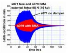
Graph showing cable oscillation (mm) vs time (s) for s071 free and s079 SMA (external force 98 N (10 kp)). The SMA damper significantly reduces the oscillation amplitude compared to the no damper case.
