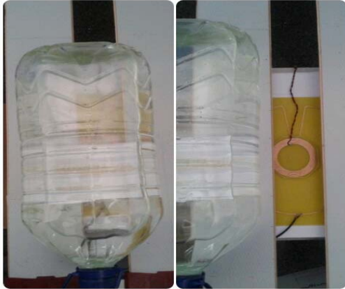
Figure 2 Experiment setup (saline solution over the sensors)
