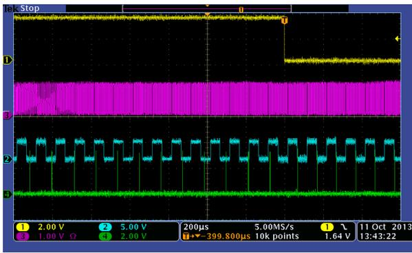
Fig. 9. Screenshot of the end of an acquisition process. From top to bottom: trace #1 is the acquisition signal, trace #3 is the QPSK-modulated signal, trace #2 is the receiver symbol clock and the trace #4 depicts the samples obtained and, indirectly, the time instants when they are obtained.
