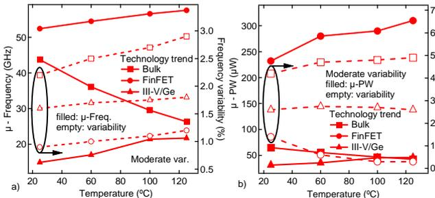
Figure 8. Impact of the environment temperature in the analyzed logic circuits, focusing on frequency (a) and PW (b), and when they are based on different technology trends and under a moderate variability scenario.
