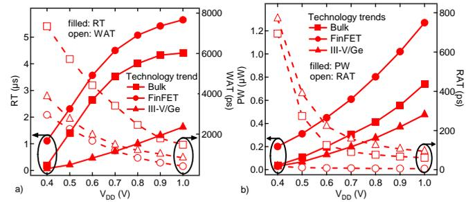
Figure 5. Impact of each technology trend on 3T1D-DRAM performance focused on RT-WAT (a) and PW-RAT (b), when  $V_{DD}$  is swept (0.4–1 V).
