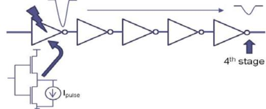
Figure 2. Schematic of the soft error analysis. The shrink of the propagated pulse illustrates the electric masking of each technology trend.
