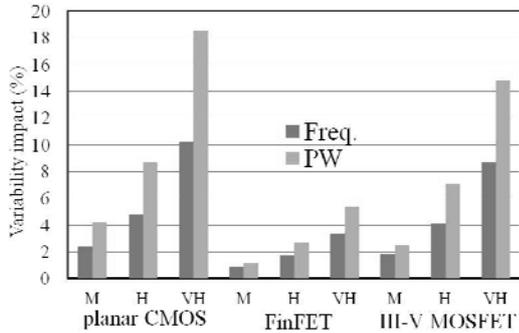
Figure 7. Variability impact on ROSC circuits for the three fluctuation levels considered, i.e. moderate (M), high (H) and very high (VH).
