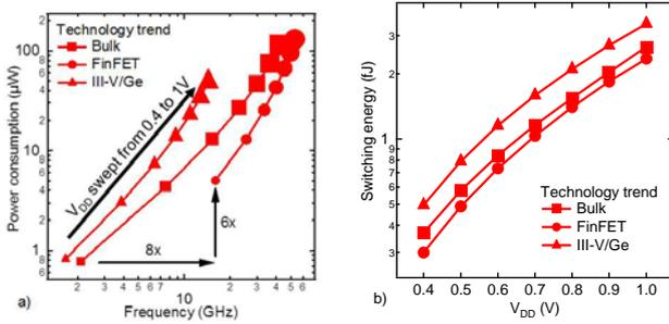
Figure 3. Relevance of the technology trend, i.e. bulk (square), FinFET (circles) and III-V/Ge (triangles), in ROSC under different scenarios: a) Relation between dynamic power consumption and operating frequency of the analyzed ROSCs. b) Switching energy as  $V_{DD}$  is reduced.
