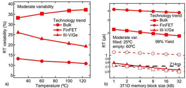
Figure 10. Impact of the environment temperature on 3T1D cells under a moderate variability scenario (a), and memory block (b).
