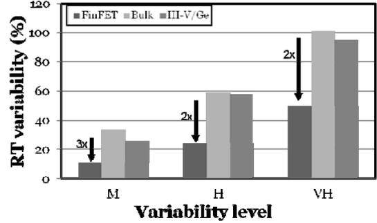
Figure 9. Impact of the process variation on 3T1D-DRAM cells, when it is subjected to different variability levels, i.e. moderate (M), high (H) and very high (VH).
