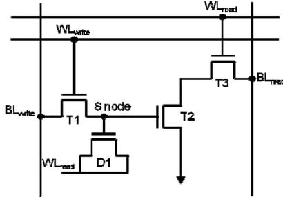
Figure 1. Schematic structure for a 3T1D-DRAM memory cell, where WL is wordline and BL is bitline.
