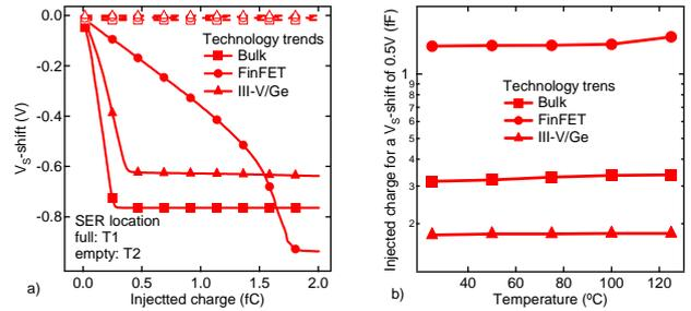
Figure 12. a) Impact of the injected charge in the storage node of the 3T1D cell at  $V_{DD}=1$  in a write-read cycle, a reduction on  $V_S$  is observed. b) Negligible influence of environment temperature into the  $IC_{min}$  is observed.
