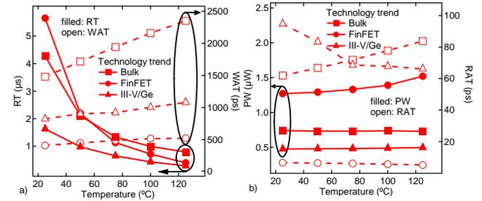
Figure 6. Impact of each technology alternative on 3T1D-DRAM performance measured as RT-WAT (a) and PW-RAT (b), when environment temperature is swept up to 125°C.
