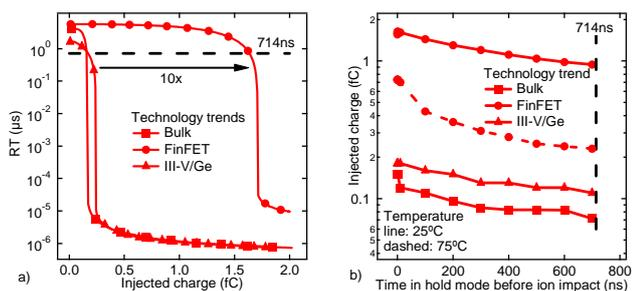
Figure 13. a) Reduction of RT in hold mode when a SER impact in the storage node of the 3T1D cell at  $V_{DD}=1$ . b) Influence of SER in hold mode for a logic 1, longer the time, the smaller the injected charge required to upset the node. In this context, temperature relevance (dashed lines) is also analyzed, but the IC reduction is similar for all technologies, and it is related to the high temperature influence in RT.
