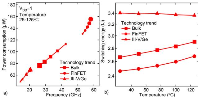
Figure 4. Impact of the environment temperature on ROSCs PW and frequency (a) and switching energy (b), when they are based on bulk (squares), FinFET (circles) and III-V/Ge (triangles).
