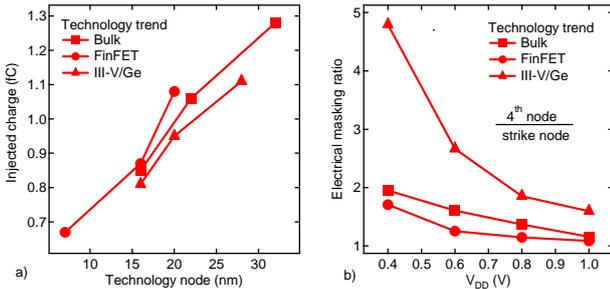
Figure 11. a) Minimum amount of injected charge required to trigger an upset event as device dimensions are reduced. b) Study of the electrical masking relevance in function of the different technology trends.
