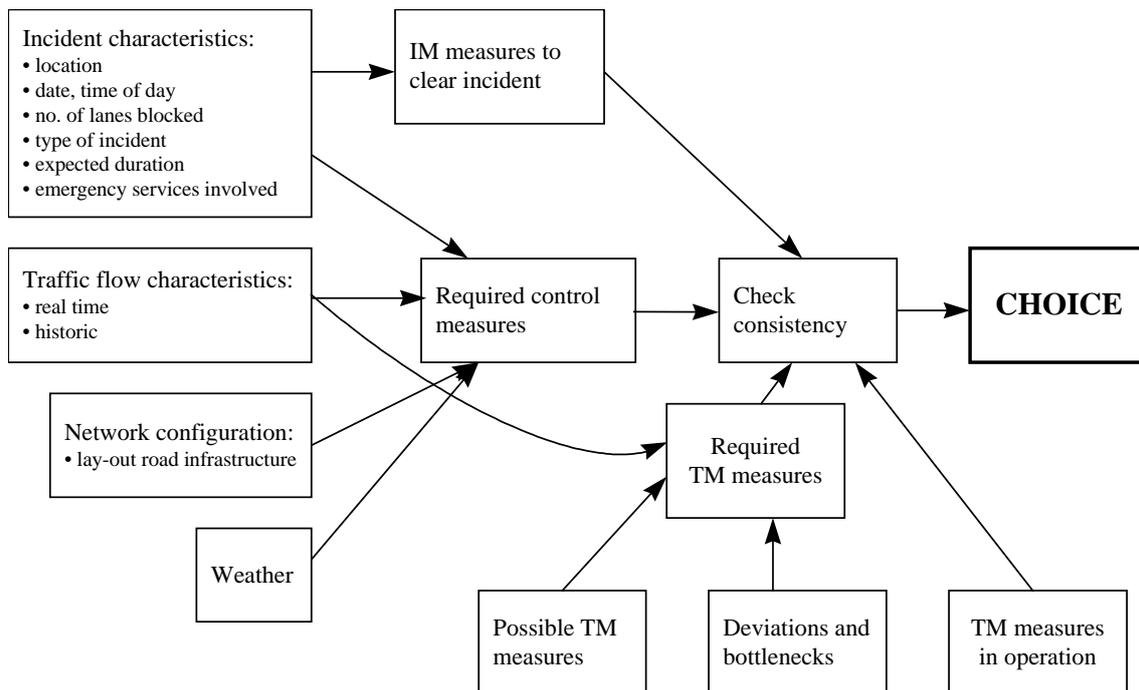
**Figure 1** Scheme of the IM and TM consistent approach
