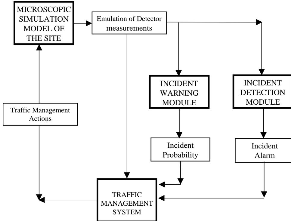
**Figure 2.** Metodological scheme for the simulation of incidents and incident management
