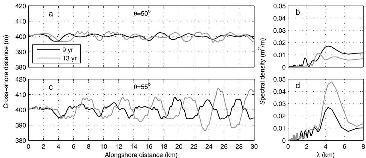
**Figure 6.** (a, c) The shoreline at  $t = 9$  and  $13 \text{ yr}$  for  $\theta_0 = 50^\circ$  and  $55^\circ$  with (b, d) the corresponding Fourier analysis of the shorelines. The shorelines can be compared to the default experiment with  $\theta_0 = 60^\circ$  in figure 3.
