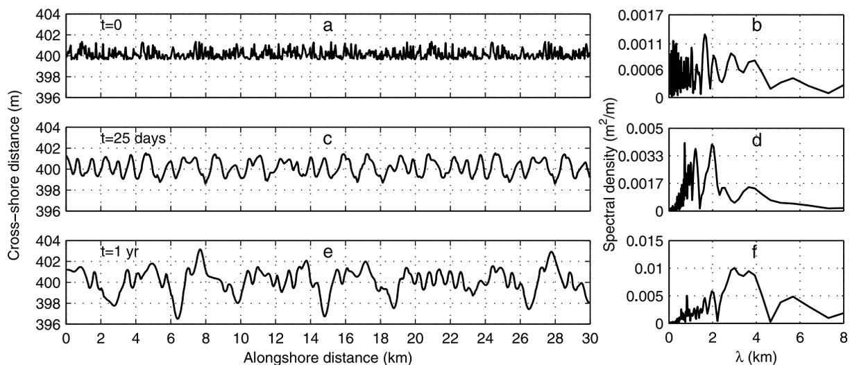
**Figure 2.** Shoreline evolution for the default experiment during the first year, showing (a, c, e) the initial development of shoreline instability and (b, d, f) the corresponding Fourier analysis of the shoreline. The waves come from the left in the plot and the cross-shore distance is exaggerated by a factor of 600.
