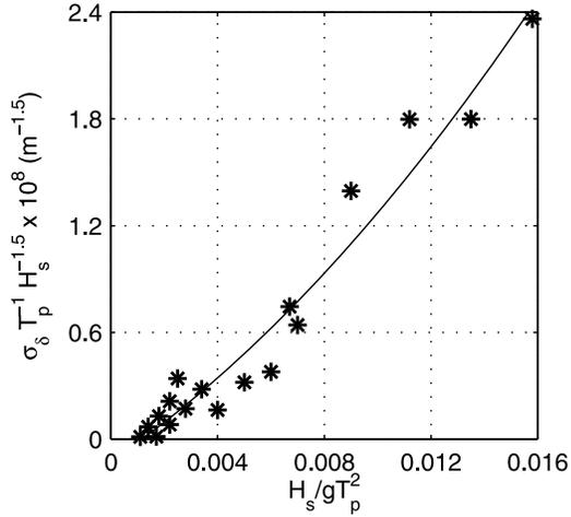
**Figure 8.** The initial growth rate of the shoreline sand waves ( $\sigma_\delta$ ), scaled with  $T_p H_s^{1.5}$ , as a function of  $H_s/gT_p^2$ . The solid line is a second order polynomial fit with  $R^2 = 0.96$ .
