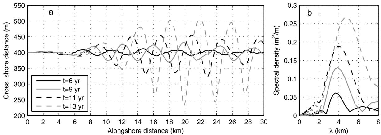
**Figure 3.** Shoreline evolution between 6 and 13 years, showing (a) the growth and migration of a regular sand wavefield and (b) the corresponding Fourier analysis of the shorelines. The waves come from the left and the cross-shore distance is exaggerated by a factor of 40.
