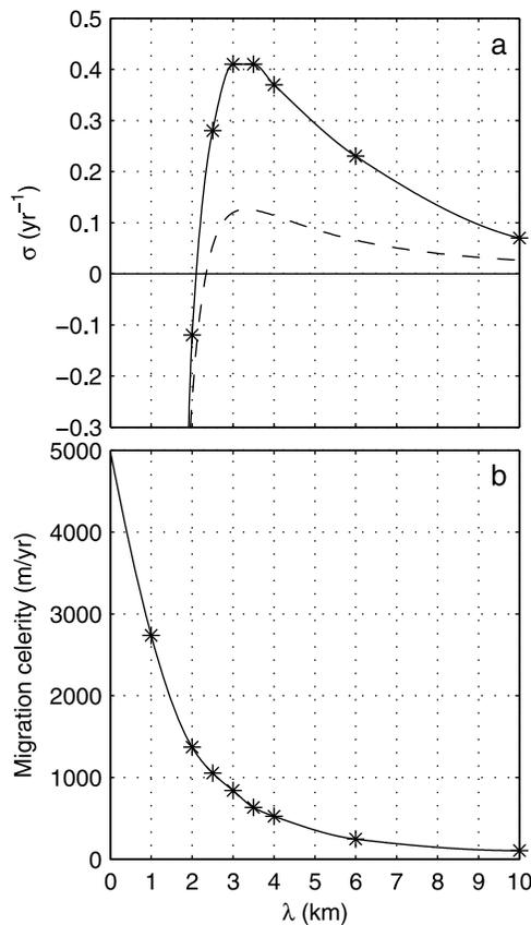
**Figure 9.** (a) The average growth and (b) migration rate of the sand waves of an initially undulating shoreline as a function of the wavelength of the undulations for default conditions. A negative growth rate indicates diffusion of the sand waves. The dashed line in Figure 9a is the growth curve computed with the linear stability model of *Falqués and Calvete* [2005] for similar conditions. The symbols indicate the data points associated with the simulations.
