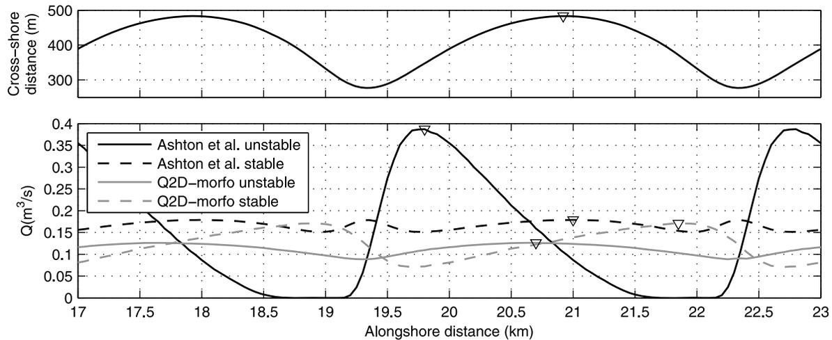
**Figure 13.** (top) The shoreline position of an undulating coast with  $\lambda = 3$  km. (bottom) The alongshore distribution of the sediment transport rate computed with the equation of *Ashton et al.* [2001] ( $Q_\infty$ ) and computed with Q2D-morfo (similar to Figure 12) for stable and unstable conditions. The symbol  $\nabla$  indicates the maxima of the shoreline position and the alongshore transport.
