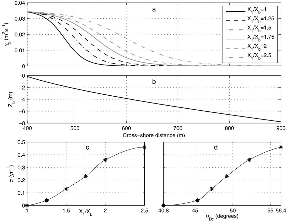
**Figure 7.** (a) Cross-shore diffusivity profiles as a function of  $X_1/X_b$  ratio. (b) The equilibrium beach profile. (c) Growth rate of the shoreline sand waves as a function of  $X_1/X_b$  and (d) growth rate as a function of the wave angle at the ‘depth of closure’ corresponding to each diffusivity profile.
