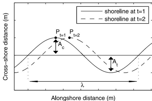
**Figure 4.** Definition sketch of a shoreline sand wave, where  $A_c$  is the amplitude of the crest,  $A_t$  is the amplitude of the trough,  $\lambda$  is the wavelength and  $P_t$  is the position of the crest. The mean amplitude is  $\bar{A} = (A_c + A_t)/2$  and the migration celerity is  $v = (P_{t=2} - P_{t=1})/\Delta t$ .
