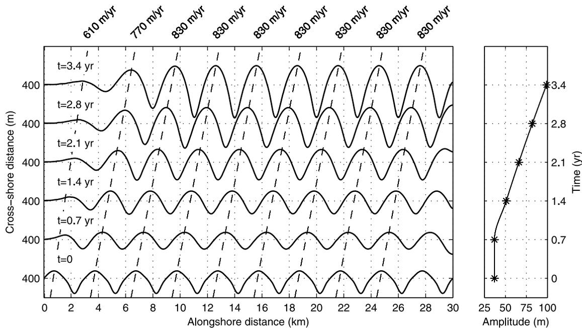
**Figure 10.** Uniform evolution of an undulating shoreline with an initial wavelength of 3 km for default conditions ( $\theta_0 = 60^\circ$ ). The migration celerity of the sand waves is indicated by the dashed lines and the growth of the mean amplitude is plotted in the right panel.
