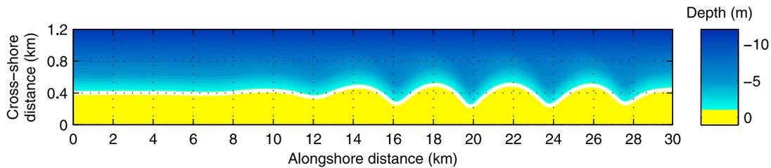
**Figure 5.** Contour plot for the default experiment showing the bathymetry after 13 years. The cross-shore distance is exaggerated by a factor of 4 and the waves come from the left.
