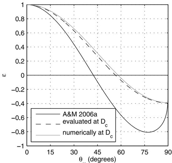
**Figure 11.** The shoreline diffusivity,  $\epsilon$ , as a function of the deep water wave angle after *Ashton and Murray* [2006a] (solid line). The deep water angle dependance of  $\epsilon$  evaluated at  $D_c$ , refracted back to deep water quantities (dashed line). The angle dependance of  $\epsilon$  computed numerically at  $D_c$ , refracted back to deep water quantities (gray line).
