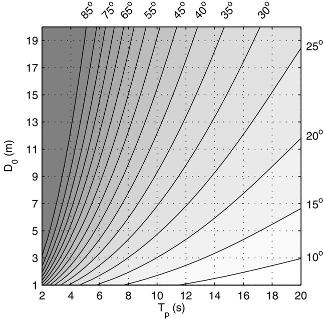
**Figure 1.** Maximum allowed wave angle at water depth  $D_0$  as a function of wave period,  $T_p$ . A deep water angle  $\theta_\infty = 89.9^\circ$  is assumed at a water depth  $D_\infty = 250$  m.
