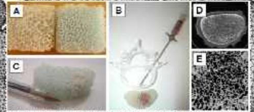
Figure 1. A. Synthetic polyurethane open cell rigid foams; B and C. Bone cement injected into synthetic foam; D and E.  $\mu$ -CT and 3D reconstruction of a ROI sample of human lumbar vertebral body.
