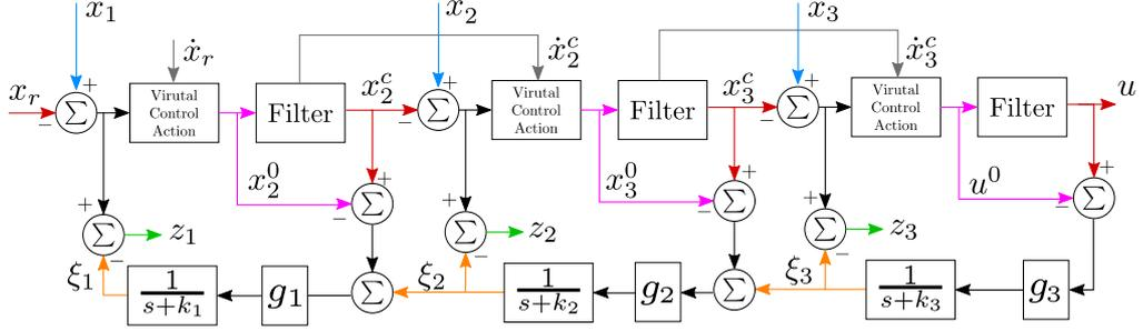
Fig. 1. Backstepping controller arrangement. Colours has been added to highlight the pattern repetitiveness in the construction.
