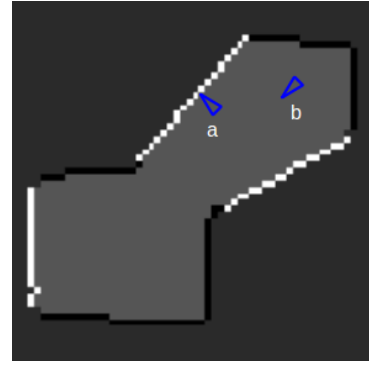
Fig. 4. Pose a : Frontiers method's exploratory goal. Pose b : Optimal map entropy reduction goal in C-space.
