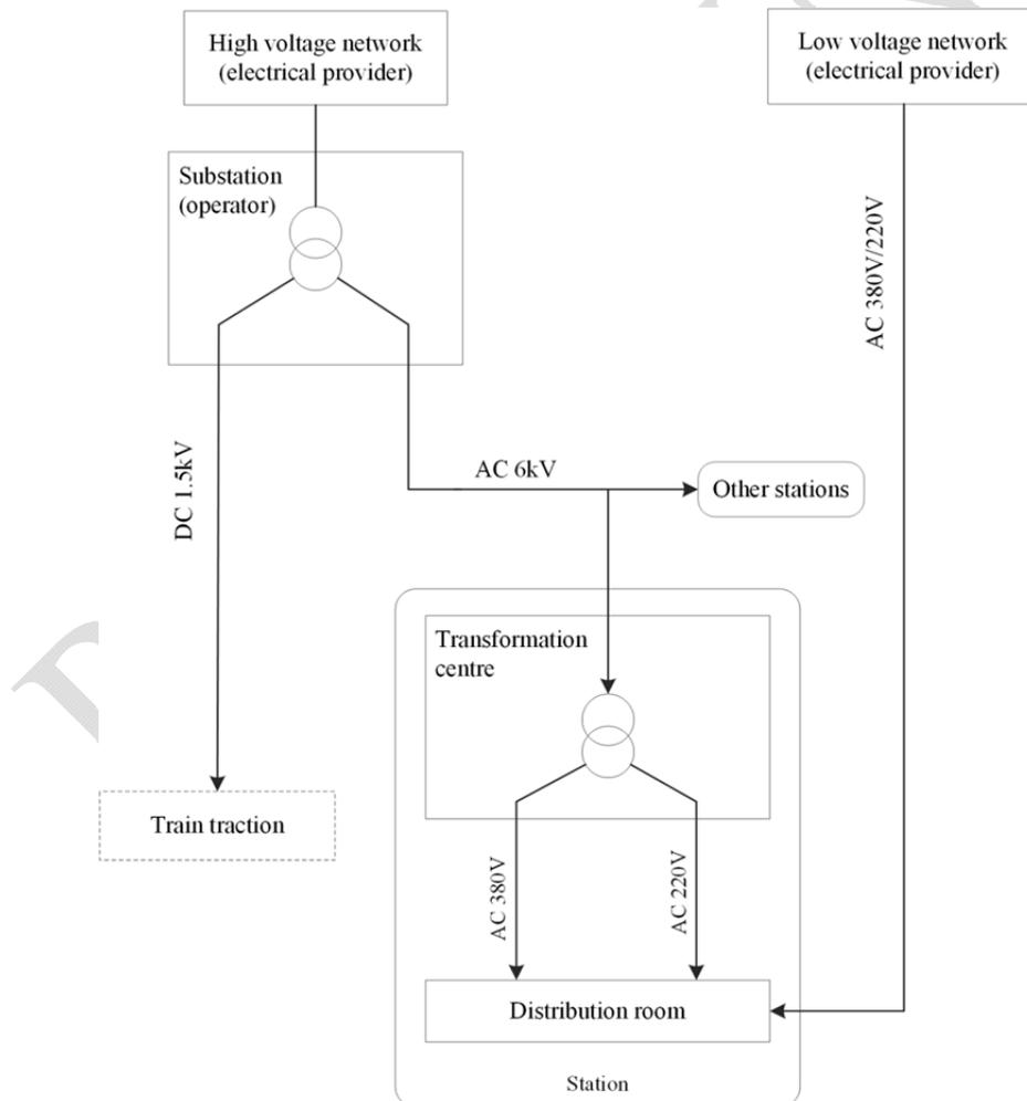
Figure 2. Power distribution in the Barcelona metro network. Source: adapted from TMB.
