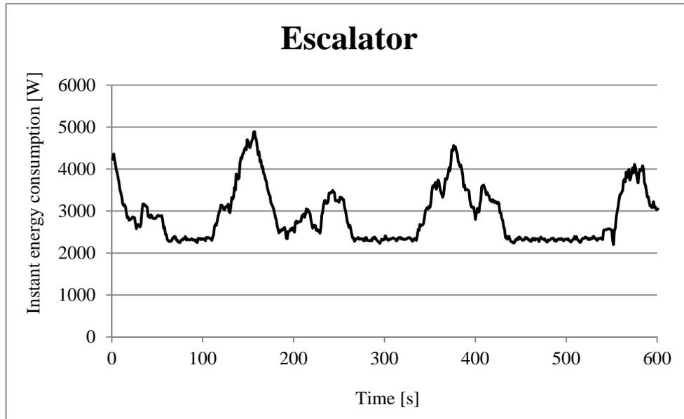
Figure 5. Instant energy consumption for an escalator running at 0.5 m/s during a 10 minute period.
