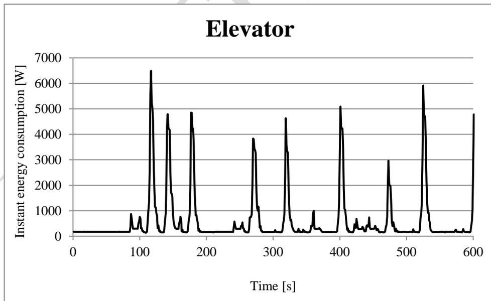
Figure 4. Instant energy consumption for an elevator during a 10 minute period.
