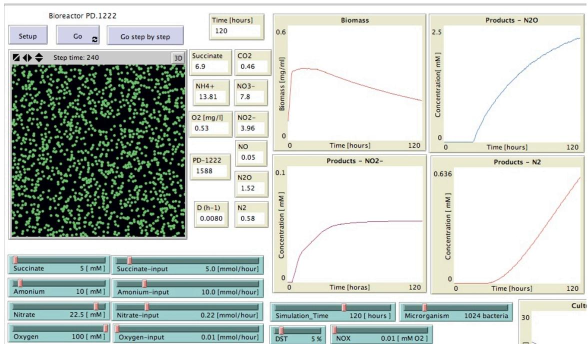
**Fig. 2.** A screenshot of INDISIM-Paracoccus simulator. Sliders to control values for the model parameters with graphical and numerical outputs.
