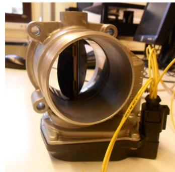
Fig. 1. Upper: throttle schematic. Lower: picture of the automotive electronic throttle body used in the experiments described in Section III.
