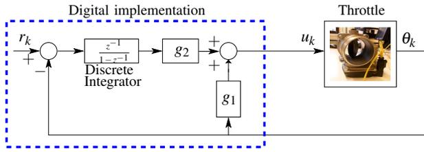
Fig. 3. Block representation of PI strategy used to control the angular position of the automotive electronic throttle body.
