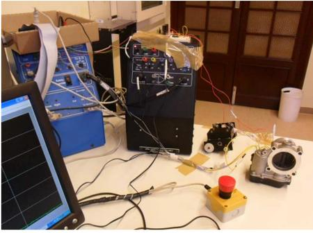
Fig. 2. Real-time laboratory testbed used to control the valve position of the electronic throttle body, according to the experimental setup described in Section III.
